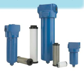
Finite's J-Series is designed to filter contaminants such as rust and pipe scale, compressor lube oil, and water from compressed gases. These filters are often used in high pressure compressed natural gas (CNG) systems, not only as inter-stage filters in the multiple stage compression of the gas, but also in the storage and delivery of the gas to CNG powered vehicles.
